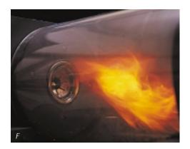
Afterburn shows in these side-byside photos (E & F). ProTek Nozzle Systems eliminate afterburn (E). Standard nozzles can't prevent afterburn (F). Afterburn causes soot and coking, often resulting in more frequent cleanings and callbacks.
